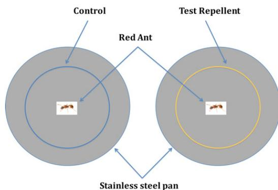
**Figure 1. Schematic of apparatus.** A stainless steel, 12-inch pan was used as the arena. For each trial, one of the non-toxic household products was deposited in a 6-inch diameter ring within the 12-inch pan. A single ant was placed at the center of the pan to commence each trial.
