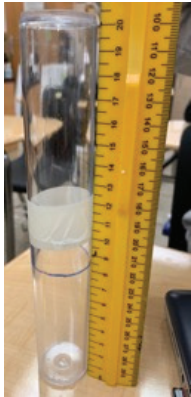
Figure 2. A picture of the negative geotaxis assay apparatus. The apparatus was constructed using two vials and masking tape. A mark at a point 8.5 cm above the bottom of the vial was made.
