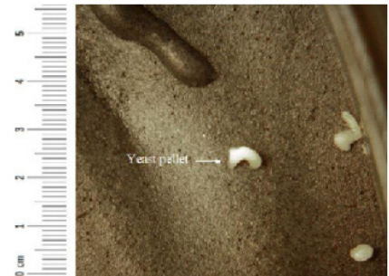
Figure 3. A photo of yeast pellets. These yeast pellets are the standard size of the pellets used in the experiments.
