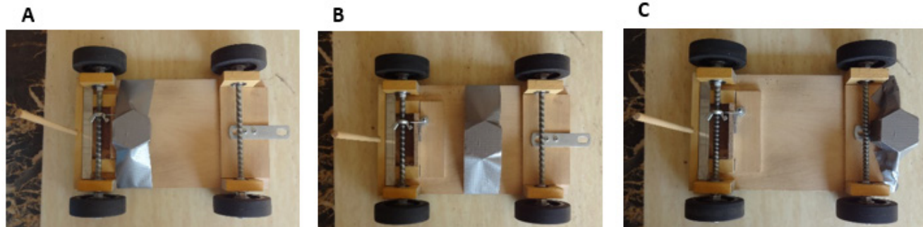
Figure 1: Gravity Vehicle with Different Mass Loading. (A) The front load was located behind the front axle due to the dowel in front of the axle. (B) The load was located at the middle point of the vehicle length, and the load behind the rear axle. All three load configurations were located on the center line and secured with duct tape to prevent movement during the run.
