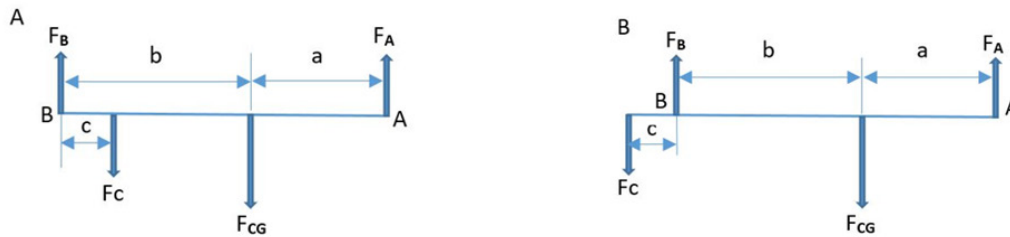
Figure 8: Diagram of Force Analysis. (A) The mass load ( F_C ) is located between the two fulcrums. F_A is the normal force from the front wheels, F_B the normal force from the rear wheels, and F_{CG} is the gravitational force at the CG. a is the distance of F_{CG} from the fulcrum A, b is the distance of F_{CG} from the fulcrum B, and c is the distance of F_C from the fulcrum B. (B) The mass load ( F_C ) is located behind the fulcrum B. All symbols are same as those of (A).
