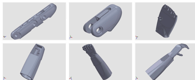
Figure 3: 3D models of various 3D prosthetic components: (a) distal phalange, (b) assembled proximal and distal phalanges, (c) palm, (d) forearm, (e) palmer aspect of assembly, (f) dorsal aspect of assembly.
