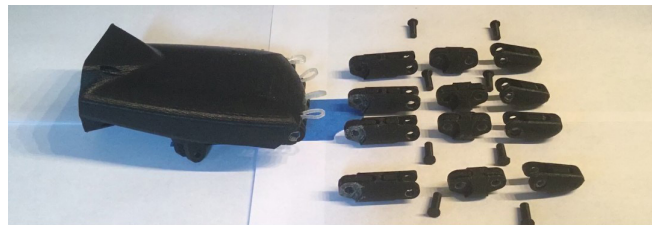
Figure 5: Unassembled 3D- printed components palm proximal, middle, and distal phalanges.
