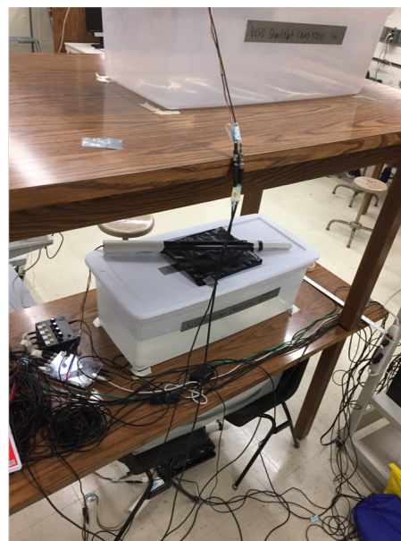
Figure 8. Detector positioning for shielding experiment. The image illustrates the actual setup of the liquid shielding flux experiment. Wire lengths and GPS positioning of each counter is entered into the data analysis software, as they affect the timing of signal reception from counter to DAQ.
