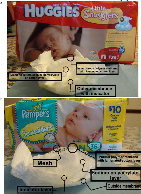
Figure 1. Cross-section of Diaper. (a) Huggies' Cross-section. (b) Pampers' Cross-section.
