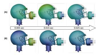
**Figure 5. Ram impact test simulation result.** (A) Titanium facemask. (B) PC1. PC1 shows less head translation by the ram impact with larger deformation. Countour shows velocity.
