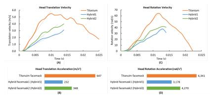
**Figure 8. Head velocity curves and head acceleration.** (A)(C) Dashed lines show linear regressions of the head velocity over 0.01 s. Hybrid1 and Hybrid2 show a slower increase of the head velocity than Titanium facemask for both the translational and rotational head velocities. (B)(D) Head acceleration comparison.
