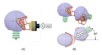
**Figure 3: Simulation condition.** (A) Ram impact test with a 5.5 m/s ram speed to the front of the helmet. (B) Helmet-to-helmet collision with a 9.3 m/s strike helmet speed with 30° attack angle.
