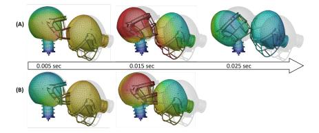
**Figure 7. Helmet-to-helmet collision simulation result.** (A) Titanium facemask. (B) Hybrid2. Hybrid2 facemask result is limited to 0.015 seconds due to a computational time constraint in the software. Angled attack generates both translation and rotation of the head. Hybrid2 facemask reduces the translation and rotation of the head. Coutour shows velocity.
