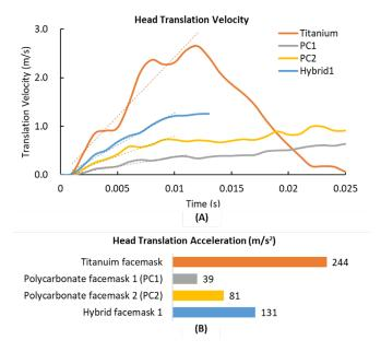
**Figure 6. Head velocity curves and head acceleration.** (A) Dashed lines show linear regressions of the head velocity over 0.01 s for each facemask. PC1, PC2, and Hybrid1 all show a slower increase of the head velocity than the Titanium facemask. (B) Head acceleration comparison.
