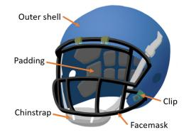
**Figure 1: American football helmet.** Facemask is mounted on the front and made of steel or titanium. Outer shell, chin strap, and clips are plastics. Padding is soft foam or rubber.
