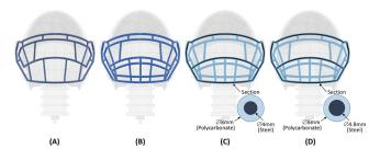
**Figure 4. Facemask designs.** (A) Titanium facemask and Polycarbonate facemask 1 (PC1). (B) Polycarbonate facemask 2 (PC2). (C) Hybrid facemask 1 (Hybrid1). (D) Hybrid facemask 2 (Hybrid2).
