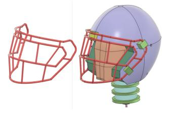
**Figure 9. Head-neck and football helmet model.** Fusion 360<sup>™</sup> model: Facemask is 3-dimensionally modeled.
