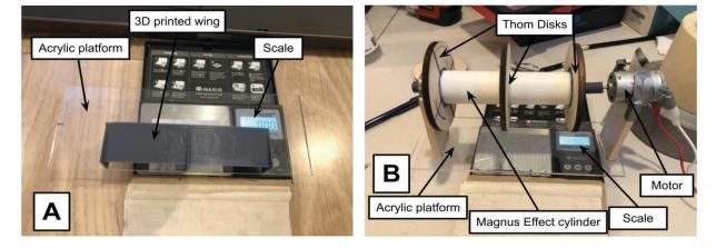
Figure 3: Pictures of the standard wing and the cylinder. (A) The front view photograph of the wing apparatus. The wing is on top of the acrylic plate which is attached to the scale. (B) The front view photograph of the cylinder apparatus. The motor spins the Thom rotor which in turn produces downforce. The cardboard buffer in front of the scale is intended to prevent airflow between the acrylic and the scale, which would produce lift.
