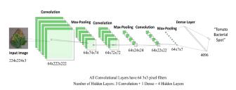
**Figure 5: Optimized shallow CNN architecture.** CNN diagram showing the setup of each layer in our optimized shallow CNN and visualizing the processing done on an example image. This architecture was determined through the hyperparameter tuning procedure.
