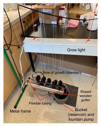
**Figure 6: Experimental setup.** This labeled image shows the entire setup of the experiment. It shows how each component was hung from the metal frame, as well as the setup of the gutter system to ensure that a consistent water flow was delivered to one end of each choice chamber.
