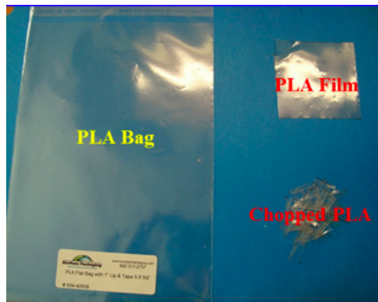
Figure 4: PLA Unchopped Films and Chopped Pieces. PLA from Nature Works LLC® used for this study. The 6x6 cm films and chopped pieces were cut from the PLA bags on the left side.
