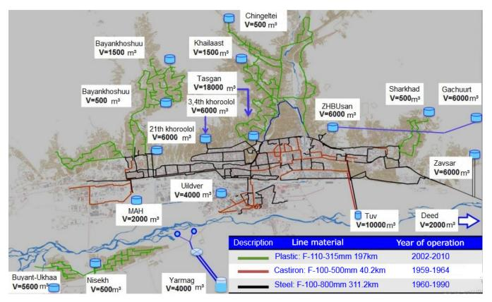
**Figure 1. Types of pipes in Ulaanbaatar City.** Blue cylinder symbols indicate the temporary storage of water supplies before being transported into the pipes. All water storages are labeled with their names. V = volume of the storage.
