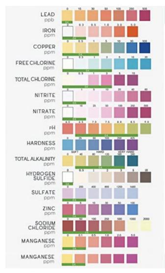
**Figure 6. Color chart for parameter testing.** The resolution guide is provided by the Varify water test kit website (16). Results were taken by comparing color change on the strips with the colors shown in this figure.
