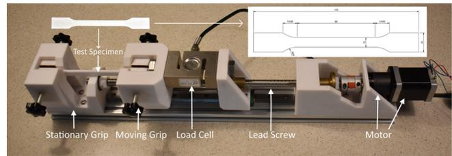
**Figure 4:** Tensile testing machine. The tensile testing machine used in this experiment is shown with the ISO 527-2 Model 1A testing specimen inserted on the left. The top right photo shows the dimensions of the testing specimen in millimeters.
