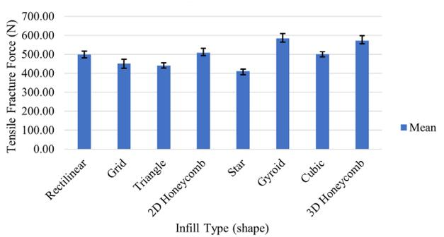
**Figure 2:** Means for each infill type. Gyroid infill had the highest mean tensile fracture force while the star shape had the lowest. Error bars indicate the range of tensile forces for each infill pattern. An ANOVA analysis showed a *p*-value of 3.3405E-18.
