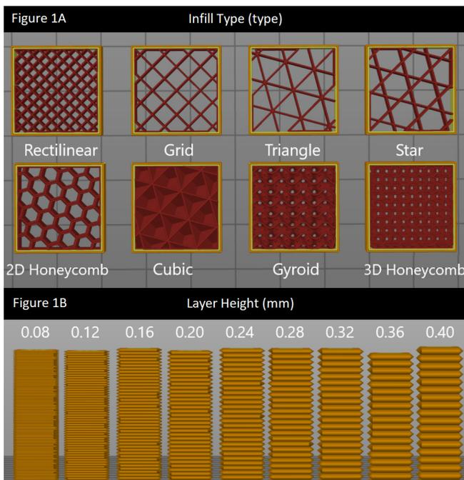
**Figure 1:** Infill patterns and layer heights. (A) Different infill patterns printed in the XY-direction and (B) different layer heights printed in the Z-direction used in this experiment to determine tensile fracture force.
