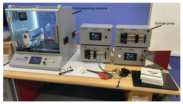
Figure 2: Spinbox Electrospinning machine with syringe pumps, which are the two boxes with metal rods and black syringe holders on their front plate. The syringe is inserted in these holders and the pump is programmed to slowly compress it, to have the fluid travel out from the syringe to the electrospinning machine on the left, where it flows out of a needle and is pulled towards the metal cylinder through a large voltage, e.g. 15 kV.
