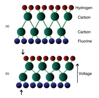
Figure 1: Beta-phase of PVDF, presenting piezoelectric properties. a) The atom arrangement structure of PDVF without applied force. b) The structure deformed by an external force applied to it, leading to a produced voltage.
