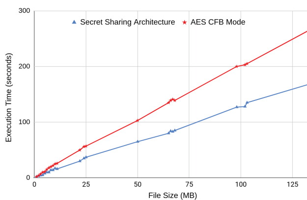
Figure 4. Performance Comparison of Document Reconstruction from Shares with a (2, 3) Scheme. To decrease sampling variability, each datapoint is the average of 10,000 individual trials of reconstructing a document of a given file size. Compared with AES, the secret sharing implementation is about 36% faster for reconstructing a document from its shares.
