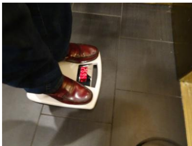
Figure 4: Measuring the change in weight due to the vertical acceleration.
