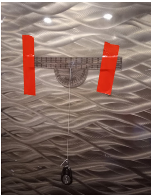
Figure 5: Measuring the deviation angle between the vertical line and the direction of the total acceleration (with gravity).
