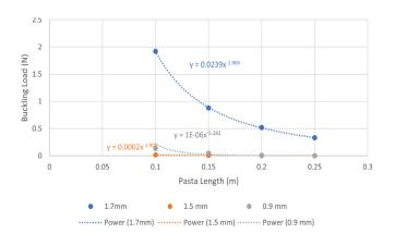
Figure 2. Buckling load (N) decreased with pasta length (m). Buckling load measured using homemade system for spaghetti-like pasta of three diameters for four spaghetti lengths. Data points are fitted with a power function and a line of best fit has been drawn for each diameter (mm).
