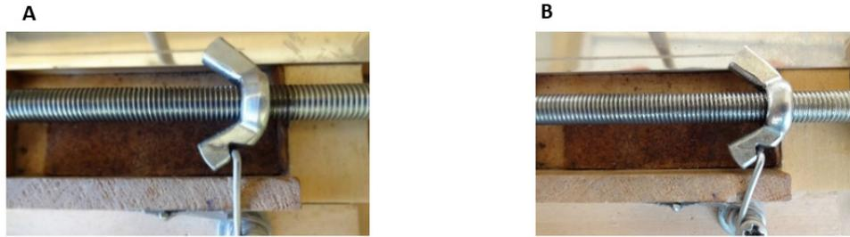
**Figure 6:** Braking System Composed of Wingnut Geared with Torsion Spring at a Specific Point. (A) The vehicle decelerates when the wingnut starts to gear with the torsion spring. (B) The vehicle stops moving when a static equilibrium between the rotational torque of the wingnut and the twisting torque of the torsion spring is established.
