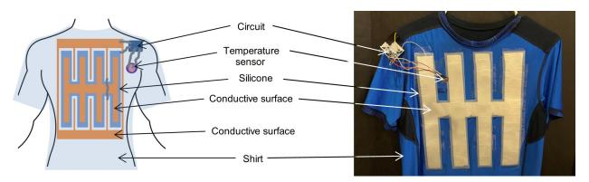
Figure 6. Diagram and image of the W-TENG. The diagram (left) and an image (right) of the W-TENG are laid out side-by-side to illustrate the different elements of the generator.
