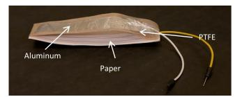
**Figure 8. Aluminum, paper, and PTFE based TENG.** This is a contact-separation mode TENG made to evaluate the effects of using different negatively charged materiasl in a TENG. In this generator, PTFE is the negatively charged material, paper is the positively charged material, and aluminum is the conductive surface.
