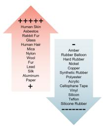
**Figure 1. Triboelectric series of various materials.** Ranking of materials by their tendency to gain/lose an electron (20). The red series indicates materials that have a more positive charge, whereas the blue section indicates materials with a more negative charge. The direction of the arrows, "+" and "-" represent a relative ranking of the materials' charge affinity.
