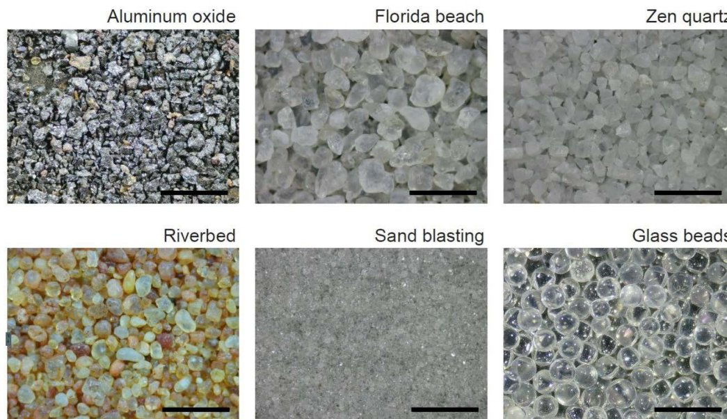
Figure 2: Microscopic images of the granular materials used in this study. Representative digital microscope images (3.0 mm × 3.5 mm field of view) are shown for each of the six granular materials examined. The black scale bar in the lower right corner corresponds to 1 mm.
