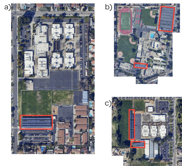
Figure 4: Tiling examples. Shown are sample outputs from the geospatial data preprocessing pipeline. Only images (tiles) intersecting the school’s assessor parcel are requested and subsequently fed into DeepSolar for PV classification, all of which were classified as positive. The methodology involved GIS-based polygon bounding and satellite image API retrieval.
