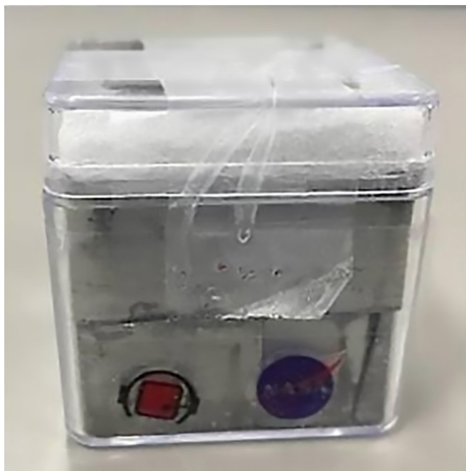
Figure 1: Packed cube experiment. A sample packet containing blood samples was placed in a plastic cube, packed with foam to protect against vibrations, and lined with lead foil to combat radiation.
