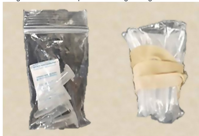
Figure 6: Sample packet contents and wrapping technique. Packet contained four microcentrifuge tubes filled with dried blood and blood plasma and one desiccant pack, all sealed in a bag tied with an elastic band to conserve space in the cube.
