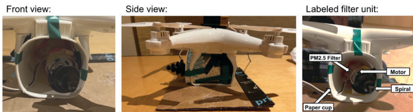
Figure 3: Materials and assembly of the filter unit. To make the filter unit inexpensive, these materials were found around the house and used for initial testing. The spiral, motor, and cup are assembled to create the cleaning function of the data processing and transmission system. This part of the system will be triggered by a signal sent between the Arduinos and has been proven effective in cleaning polluted air (17).
