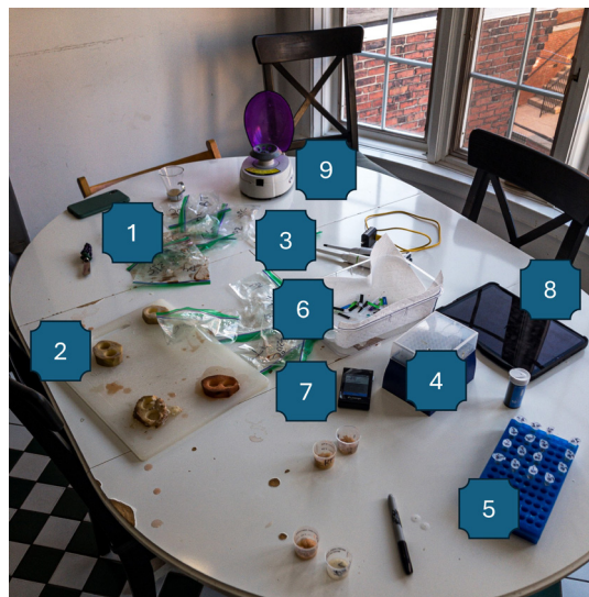
Figure 3. Select equipment and consumables used in the study. 1) Ziploc bags; 2) potato slices; 3) 1,000- \mu l automatic pipettes; 4) pipette tips; 5) 1.5-ml Eppendorf tubes; 6) glucometer testing strips; 7) – glucometer; 8) iPad; 9) mini-centrifuge. Not shown: Anova immersive circulator and garlic press.
