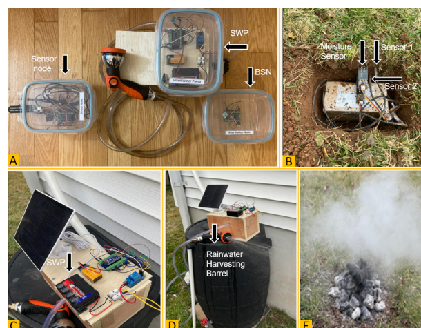
Figure 2: Field testing setup. A) Sensor node, SWP and BSN components. B) The sensor node was installed under the soil with Sensor 1 and the moisture sensor placed at a one-inch depth and with Sensor 2 placed at a three-inch depth. C) A SWP was installed with D) a harvested rainwater barrel. E) On detecting rising soil temperature and moisture levels, the BSN triggered the SWP to extinguish the fire.
