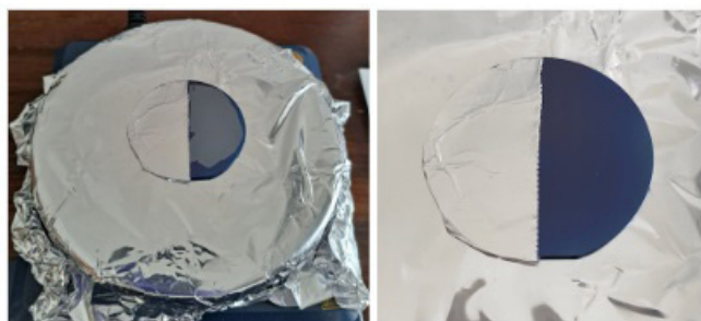
Figure 2: APTS coating on a silicon wafer. The image shows the process of APTS coating on a hot plate. Half of the silicon wafer was covered using aluminum foil (left) while the other uncovered half of the wafer was coated with APTS (right). The half-wrapped silicon wafer was placed onto a hot plate at 100°C and the right side was coated with 25 g of 95% APTS for 5 minutes. The wafer was then rinsed with pure acetone and air-dried.
