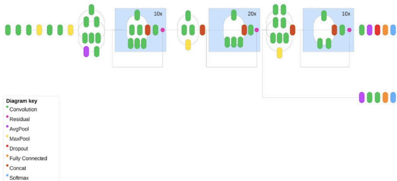
Figure 1: Figure 1. Schematic Diagram: Compressed View of Base Neural Network Inception-ResNet-v2. The authors used LucidChart software to model the Inception-ResNet-v2 architecture. The various blocks represent different components of the architecture: green represents convolution layer, pink for residual connections, purple for the average pooling layer, yellow for the max pooling layer, red for the dropout layer, orange for fully connected layer, brown for the concatenation layer, and blue for the SoftMax layer. The light blue boxes represent the sizes of the convolutional filters used in the depthwise separable convolution blocks.
