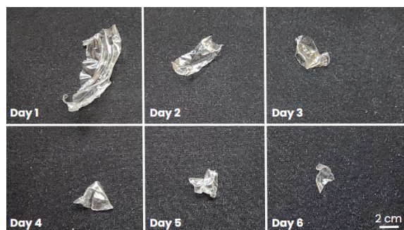
Figure 4. Biodegradability of sodium alginate composite films. Volume reduction after six days in microbial conditions. A composite film was submerged in a plot of soil and observed daily. After seven days in microbial conditions, the film completely degraded.
