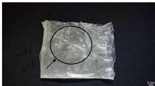
Figure 5. Sodium alginate film with blended calcium chloride. Sodium alginate film with 2 mL of 0.1% (w/v) calcium chloride blended into it. The calcium chloride solution was mixed at 1500 rpm for 30 minutes to produce this film. The resulting film displayed inconsistencies in its transparency in the form of white spots.
