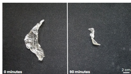
Figure 2. Volume reduction from water submersion. Representation of one sample degrading over 90 minutes as a result of water submersion. The sample was submerged in 100 mL of distilled water, with periodic check-ins every 90 minutes. Complete hydrolysis was achieved in 180 minutes.
