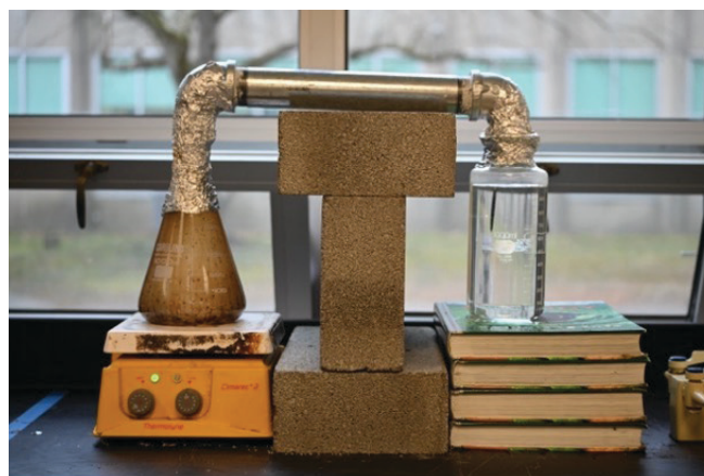
Figure 4: Smoke solution system. A flask, which contains the plant material, is located on a hot plate (left). A tube from the plant container connects to a beaker with 1 L distilled water (right). The system is sealed with aluminum foil to prevent any gas from escaping. Smoke from the heated plants will dissolve into the water in the water beaker.
