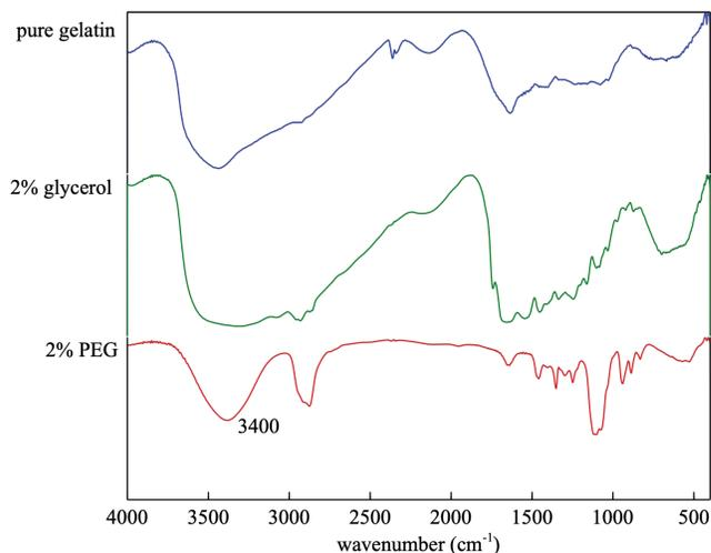
**Figure 5: FTIR of gelatin biofilms.** FTIR spectrum of pure gelatin film, 2% w/v glycerol film and 2% w/v PEG film. Samples of gelatin films were tested with a wavenumber of  $400\text{ cm}^{-1}$  to  $4000\text{ cm}^{-1}$ .
