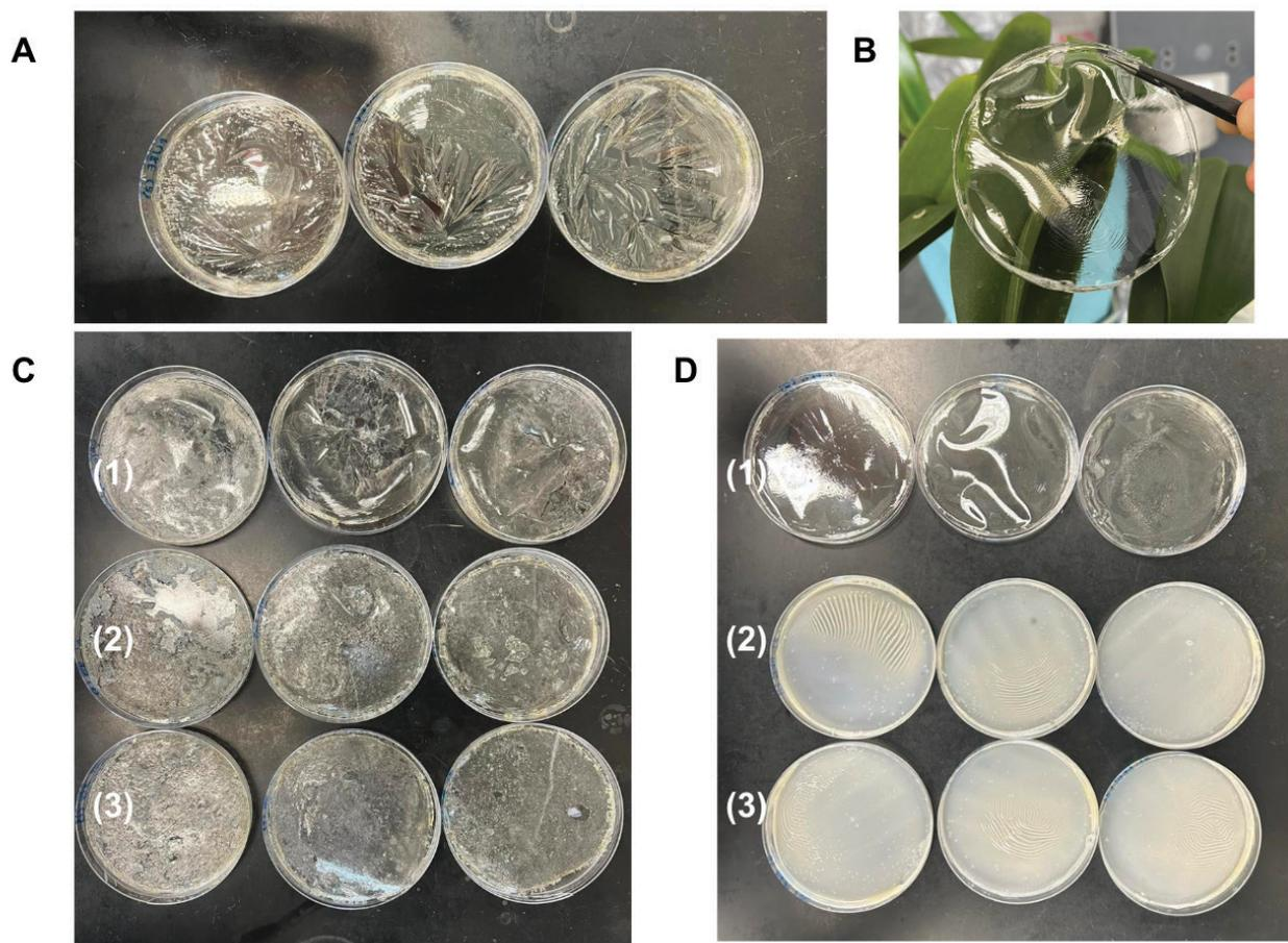
**Figure 1: Qualitative observations of the dried biofilms.** Gelatin films were dried in Tryptic Soy Agar Petri dishes at 60 °C in an oven for 24 hours. Photographs of dried (A) pure gelatin, (B) Film of 1% w/v PEG concentration against a houseplant to demonstrate transparency, (C) glycerol plasticized, and (D) PEG plasticized films. In C-D concentration (w/v) is indicated on each row where (1) = 1%, (2) = 2%, and (3) = 3%.
