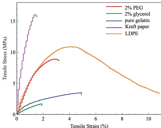
**Figure 4: Stress-strain analysis.** Tensile strain against tensile stress of pure gelatin films, 2% w/v glycerol and PEG films, LDPE and Kraft paper. Film samples were tested using a tensile machine at a crosshead speed of 5 mm/min.
