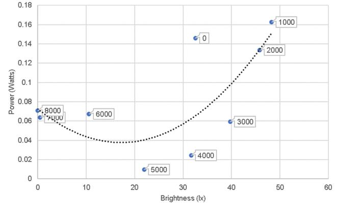
**Figure 7: Graph indicating the relationship between the brightness of the light bulb and power consumption in Room Test 4 for AC lighting systems.** Phase delay is represented by data point callouts. BH1750 sensor measured the brightness of the bulb in a completely dark room. Three sets of readings of the bulb's voltage were taken and its brightness at a particular phase delay. The dotted line represents a quadratic line of fit with  $R^2 = 0.52$ .
