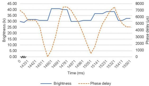
**Figure 6: Graph indicating circuit and light sensor response for AC lighting systems when the target brightness was set to 33.00 lx in Room Test 3.** An ambient room lighting of 30.00 lx was set at start of the test. This test simulated partial sunlight. The room brightness stabilized at 32.50 lx after 15 s. Inconsistent room lighting and communication time between the Arduino and the sensor caused the peaks and drops in phase delay.
