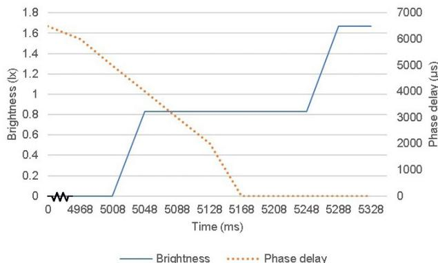
**Figure 4: Graph indicating the circuit and light sensor response for Room Test 1 for AC lighting system in complete darkness.** Complete darkness (0.00 lx) was created by switching off the room lights. Next, the transformer was switched on and the light was observed to switch on and reach its maximum brightness. The least count of the BH1750 sensor used was 0.83 lx, while the brightness readings of this test were observed at 0.20 lx intervals, creating a step-like graph.
