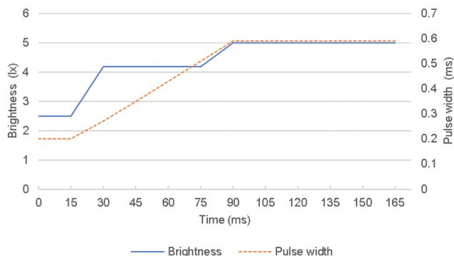
**Figure 2: Response of the light sensor and the regulator circuit in Box Test 3 for DC lighting systems.** An initial brightness of 2.50 lx was created using artificial light to simulate partial lighting in the box. Readings of both brightness and pulse width were recorded by the Arduino at 15 ms intervals.
