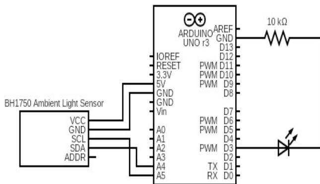
**Figure 1: Circuit diagram for Box Tests 1, 2, and 3 to regulate LED with PWM for DC lighting systems.** Brightness of the light was measured using a BH1750 sensor, while the pulse width of the LED was adjusted using the Arduino. The current passing through the LED was regulated by the resistor and also to prevent the LED from burning. Acronyms from the diagram are specified in Appendix 1.
