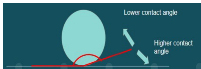
Figure 1: Explaining Contact Angle. The contact angle of a water droplet is the angle of the bottom curve to the surface of the wafer. In this figure, the contact angle is very high, suggesting that the surface is hydrophobic because it is repelling the water.
