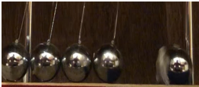
Figure 3: Image of spheres from 1 layer tape trial. The minimal separation of the body of spheres observed despite the presence of tape.
