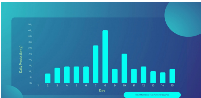
Figure 3: Average daily gas production at thermophilic temperature (60°C). Bar graph shows that the average daily biogas production is 17.57 grams, whereas the standard deviation is 9.31 grams.
