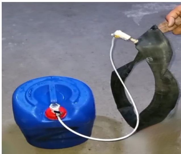
Figure 4: Digestion chamber attached with the gas collection tube. The gas collection tube is attached with the digestion chamber via an airtight pressure valve.
