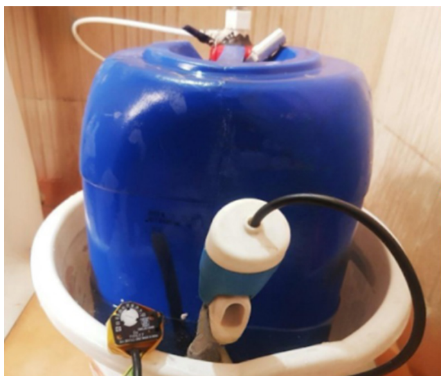
Figure 5: Waste digestion setup in a temperature-controlled water-bath. The digestion system is placed in a water bath maintaining a temperature of 60° using a thermostat along with a 250 W heating rod.
