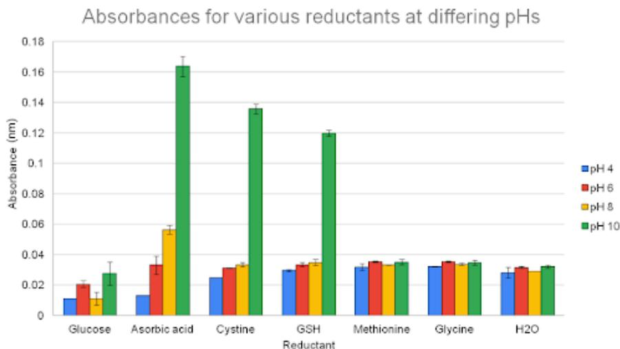
**Figure 3: The absorbances for various reductants at differing pHs (pH 4, 6, 8, and 10).** Elevated absorbance for ascorbic acid, cysteine, and glutathione at pH 10 measured at 570 nm with standard deviation error bars, suggesting their interference with the assay, and a correlation between pH and autoreduction.
