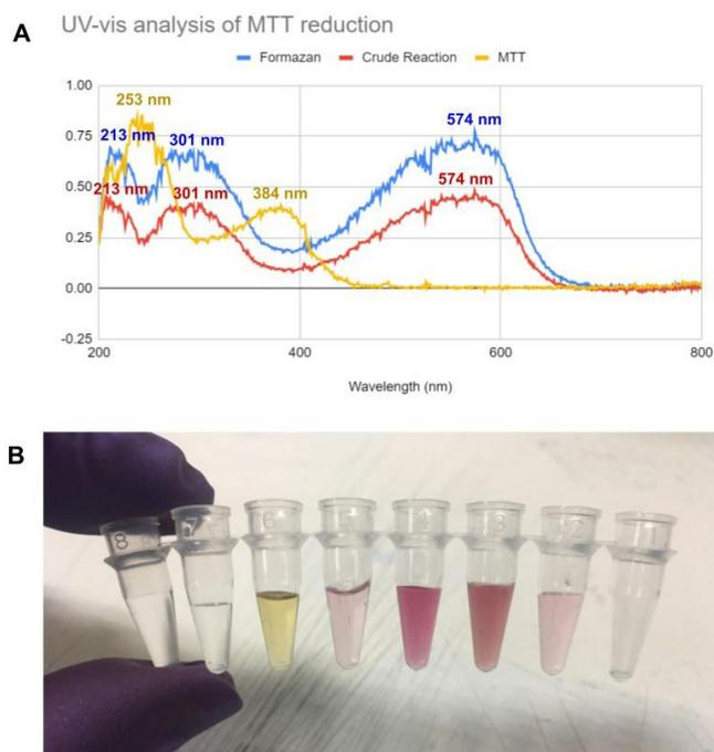
**Figure 4: UV-Vis analysis of crude reaction mixture against an authentic standard of MTT and formazan.** A) Both formazan and the crude reaction mixture had high absorbances at 213, 301, and 574 nm, suggesting that MTT is produced in this reaction. The wavelength was plotted against absorbance. B) Upon addition of base, the autoreduction reaction (exemplified: cysteine) instantaneously turns from yellow (third tube from left) to purple (right tubes).
