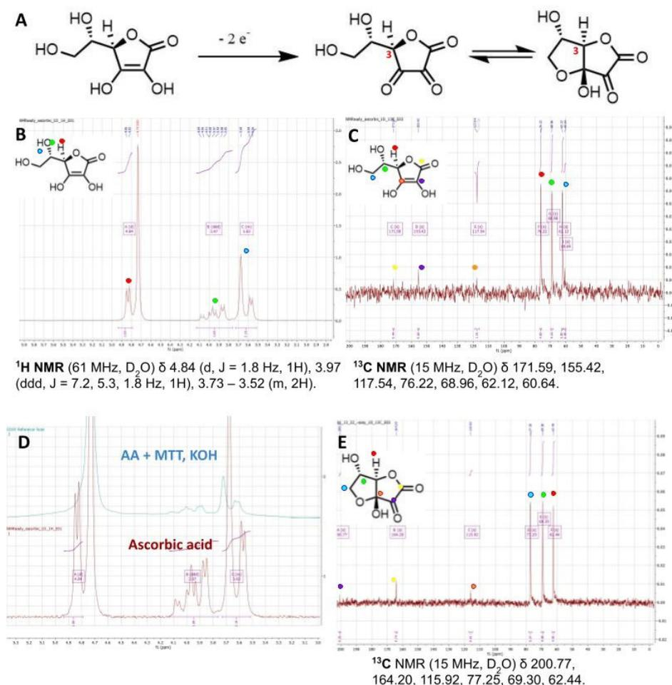
**Figure 7: NMR spectra of ascorbic acid oxidation to dehydroascorbic acid.** A) Reaction schematic for the oxidation of ascorbic acid into dehydroascorbic acid B) <sup>1</sup>H NMR of ascorbic acid C) <sup>13</sup>C NMR of reduced form ascorbic acid D) stacked <sup>1</sup>H NMR spectra of ascorbic acid (red, bottom) and reaction mixture in D<sub>2</sub>O after addition of MTT and base E) <sup>13</sup>C NMR of crude reaction mixture.
