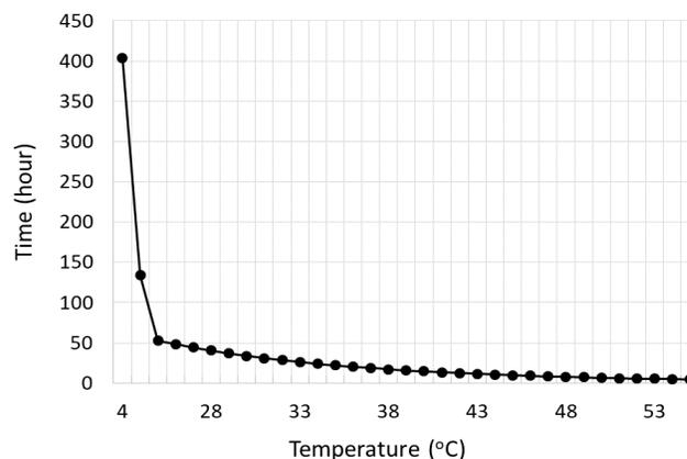
**Figure 2: Calculated shelf life of milk based on storage temperature.** The predicted time before spoilage for milk with 404-hour shelf life (17 days) at 4°C is exposed at different temperature  $T$  (°C). An activation energy of 66.7 kJ/mol was used in a model based on the Arrhenius equation (equation 1).
