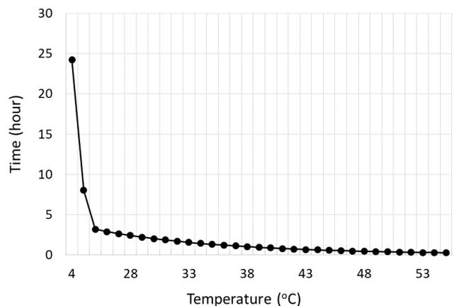
**Figure 3: Calculated shelf life of milk based on storage temperature.** The predicted time before spoilage for milk with 24-hour shelf life (1 day) at 4°C is exposed at different temperature  $T$  (°C). An activation energy of 66.7 kJ/mol was used in a model based on the Arrhenius equation (equation 1).
