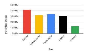
Figure 6: Overall change in temperature in each gas over all four trials. This shows the average change in temperature from the start to endpoint for each gas averaged over all four trials.
