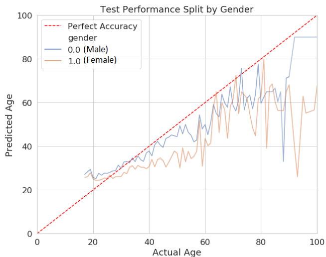
Figure 2: Accuracy of the model in terms of actual age vs predicted age when split by gender. The dataset labels “male” images with a 0 and “female” images with a 1, which was how they were separated.
