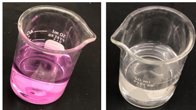
Figure 2. Color change observed due to the reaction of calcium hydroxide and carbon dioxide. Left is before reaction with the addition of phenolphthalein indicator, whereas right is after reaction.
