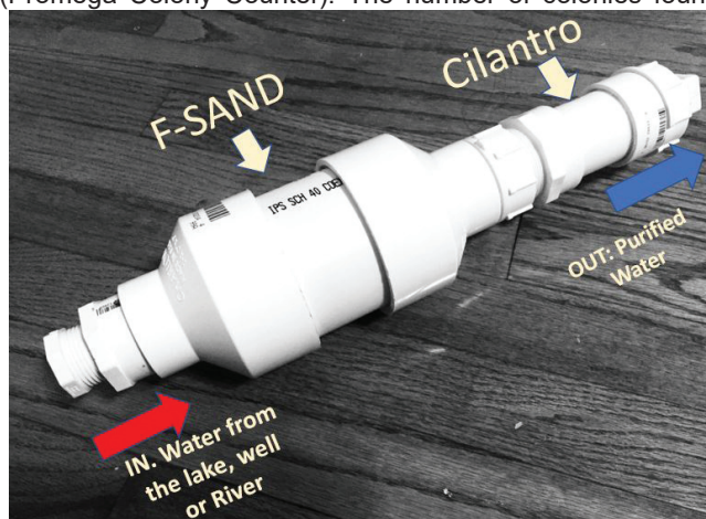
Figure 4. Filter Prototype. This is the filter prototype constructed using PVC materials there are two different components, a larger one for the f-sand and a smaller one for the cilantro.
