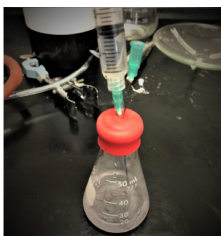
Figure 4. Nitrogen dioxide synthesis by reacting tin and nitric oxide. 0.2 g of tin was obtained, placed in a small Erlenmeyer flask and a septum stopper was placed on top of it.
