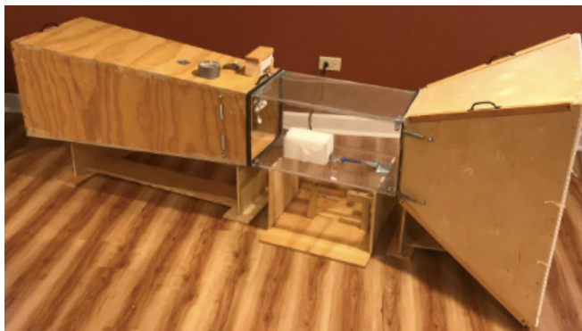
Figure 1: Wind tunnel. Completed wind tunnel with all three parts connected to one another.
