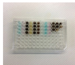
Columns (stating from left at the top) Column 1: Listerine® solution (100 \mu L) Column 2: ACT® solution (100 \mu L) Column 3: MH solution (100 \mu L) Column 4: LRE solution + Bacteria Column 5: 75% MH + 25% LRE solution (100 \mu L) Column 6: 25% MH + 75% LRE solution (100 \mu L) Column 7: Sterile Water (200 \mu L) Column 8: Listerine® solution (200 \mu L) Column 9: ACT® solution (200 \mu L) Column 10: 75% MH + 25% LRE solution (200 \mu L) Column 11 & 12: 25% MH + 75% LRE solution (200 \mu L) Column 13 (bottom right side, not shown): LRE solution (200 \mu L)
